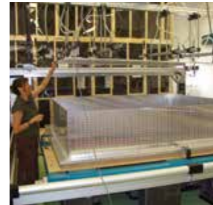
Construction of the DSECal calorimeter for T2K's neutrino near-detector.
